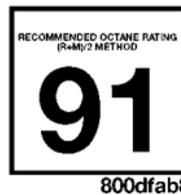
This engine is designed to meet all emissions regulations and provide excellent fuel economy and performance when using high-quality premium unleaded gasoline with an octane rating of 91.
