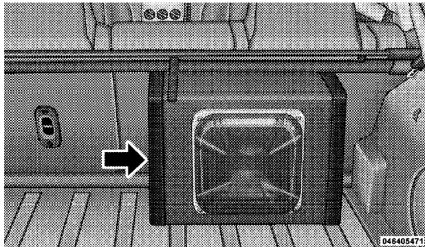
2. Slide the subwoofer toward the front of the vehicle so that the rear edge lines up with the end of the load floor.
