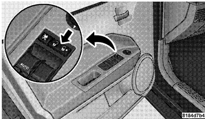
**Power Door Lock Switch Location****Automatic Door Locks — If Equipped**
