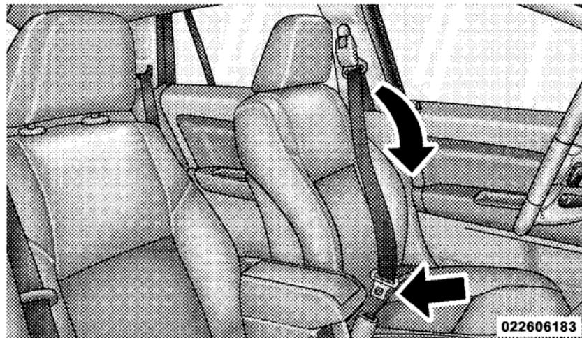
Inserting Latch Plate Into Buckle
